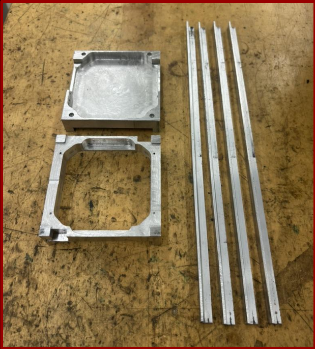
Aluminum frame components and optomechanical layer prototype made with CNC
